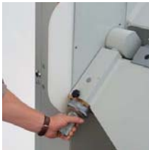
Quick folding beam material thickness adjustment, in ten seconds or less.
