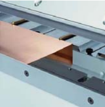
Backgauge sheet support pans are adjustable front to back, to open free space behind lower tools for pre-bent flanges going in opposite directions.
