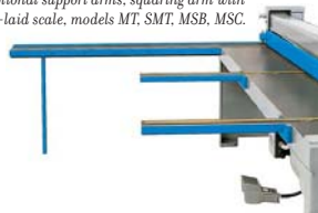
Optional support arms, squaring arm with in-laid scale, models MT, SMT, MSB, MSC.
