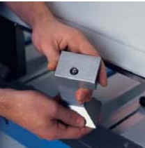
Snap-on tooling is loaded by hand, without wrenches, in seconds.
