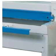
Telescoping front sheet support for large plates.
