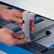
Snap-on tooling is loaded by hand, without wrenches, in seconds.
