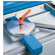
Adjustable miter gauge for miter cuts (model MSC), with scale ring (0 to 45 degrees) and clamping lever.
