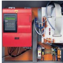
Frequency inverter powers folding beam system for extremely fast and accurate positioning.
