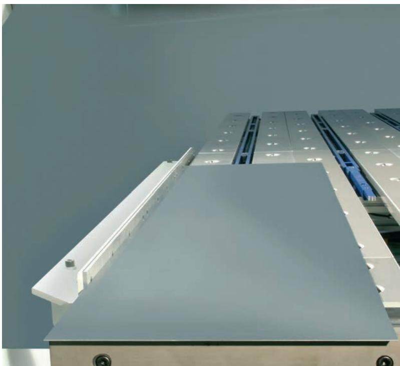
Side gauge: The precision of forming starts with an exact positioning of the workpiece.
