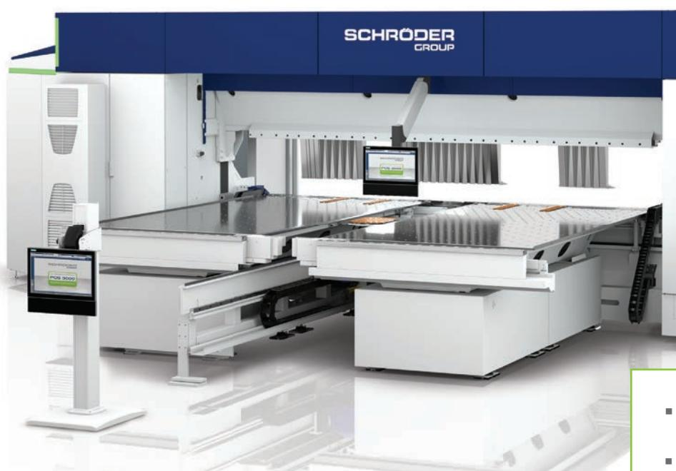
Rear view of the EVO Center with optional Advanced Handling System (AHS)
