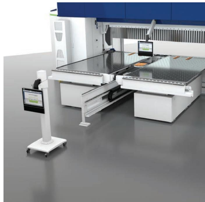
Additional operator terminal on the rear - free-standing column turnable and height-adjustable. Safety for operation from the rear: light curtain controlled by safety-PLC.
